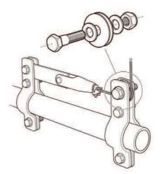
using the Grade 8.8 hexagonal M12 bolt, washers and Nylon insert nut provided. Tighten the Nylon insert nut until some thread from the bolt protrudes from end of the nut but do not tighten hard down so the sheave can still rotate slightly when subjected to a load.
